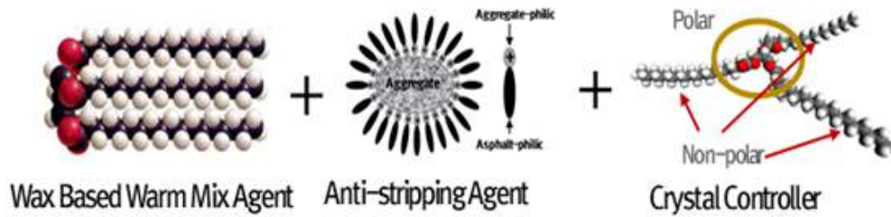
Figure 2. Composition of Korean warm-mix asphalt technology
